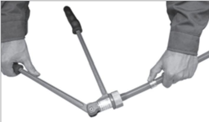
Expanding the pipe using expanding tool should be performed in three phases. First two expansions not full, then rotate the expanding tool through 30° and 15° against the pipe. The third expansion is full.
