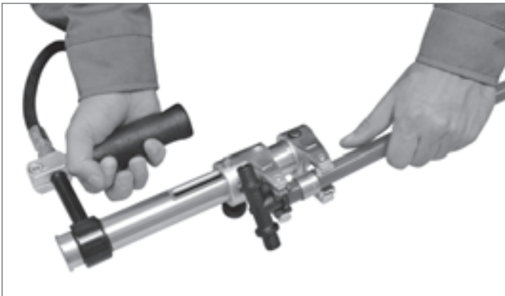
Slide the sleeve using hand or hydraulic press with foot-operated drive. Fittings can be gripped only at flanges. Do not slide two sleeves at the same time.
