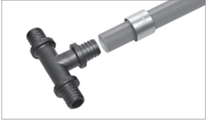
Put sleeve on the pipe with innerly beveled end from the fitting side. Carefully choose proper sleeve as there are different sleeves for pipes with and without diffusion barrier.
